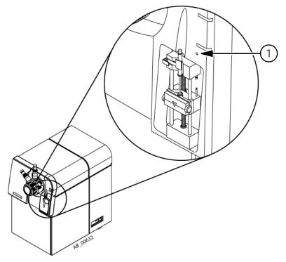
Figure 1-8 Syringe pump reset button
