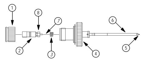
Figure 7-4 Probe - expanded view
