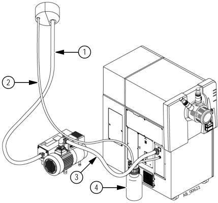
Figure 8-1 Vent connections
