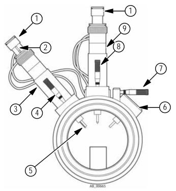
Figure 7-1 Parts of the ion source
