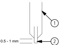
Figure 7-5 Electrode tip extension adjustment
