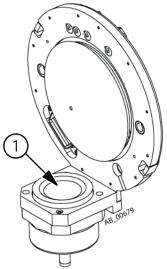
Figure 8-3 Source drain on the vacuum interface
