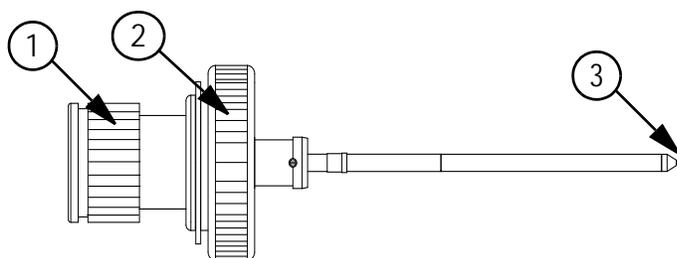
**Figure 7-3 Parts of the APCI probe**
