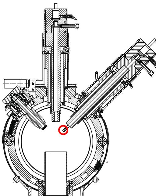
**Figure 7-6 Corona discharge needle tip at rear of ion source**
