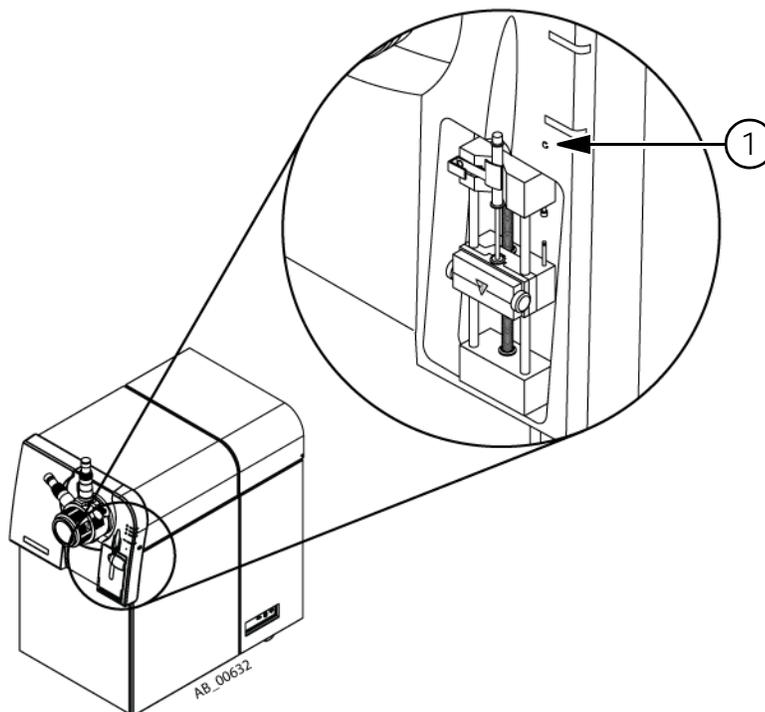
**Figure 1-8 Syringe pump reset button**
