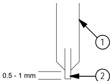
**Figure 7-5 Electrode tip extension adjustment**
