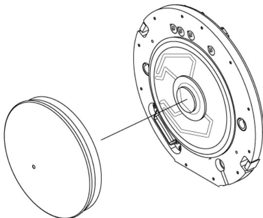
**Figure 8-4 Interface with curtain plate removed**
