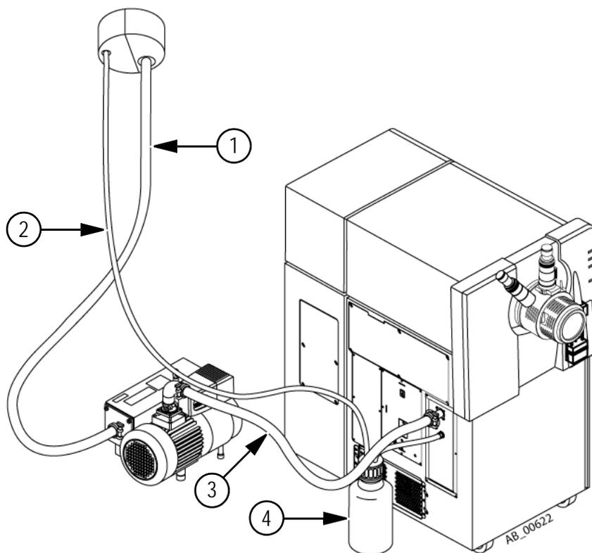
**Figure 8-1 Vent connections**
