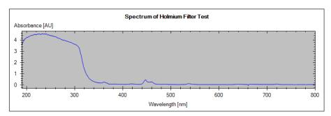
Figure 37 Holmium Oxide Test - Signals
