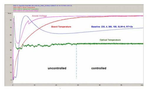
Figure 22 Detector Warm-up − 1<sup>st</sup> hour
