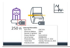
RFID tag information is displayed when moving with the mouse cursor on to the tag attached to the flow cell or lamp. The information provides flow cell and lamp related information like
