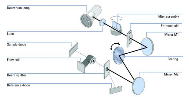
Figure 3 Optical Path of the Variable Wavelength Detector
