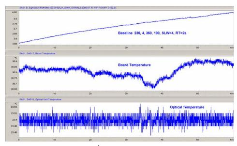
**Figure 23** Detector Warm-up – 2<sup>nd</sup> hour
