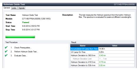
Figure 36 Holmium Oxide Test - Results
