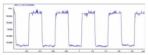
Figure 39 D/A Converter (DAC) Test – Example of Integrator Plot
