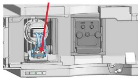
**9** Replace the fan cover (1.) and fix its screw (2.).
