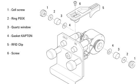
Figure 48 High Pressure Flow Cell
