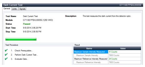
Figure 34 Dark Current Test - Results
