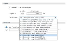
Figure 12 G7114B Peakwidth settings up to 240 Hz
