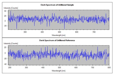
Figure 35 Dark Current Test - Signals
