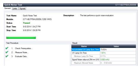
Figure 32 Quick Noise Test – Results
