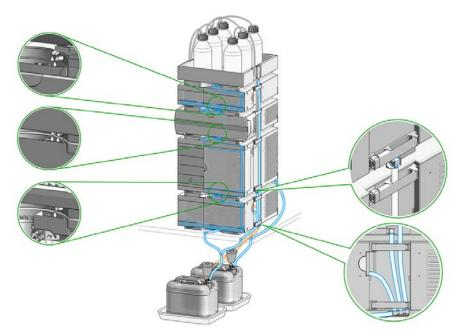
Figure 7 Infinity II Single Stack Leak Waste Concept (bench installation)
