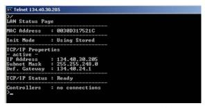
Figure 65 Telnet - Current settings in "Using Stored" mode
