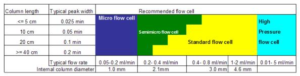
Figure 19 Choosing a Flow Cell (Standard HPLC Applications)
