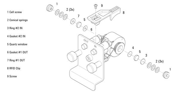
Figure 45 Standard Flow Cell
