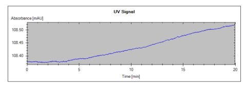
Figure 31 Drift and Noise Test – Signal
