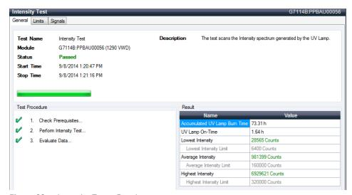
Figure 26 Intensity Test – Results
