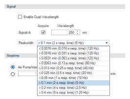
Figure 13 G7114A Peakwidth settings up to 120 Hz
