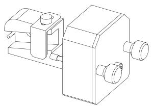
Figure 49 Cuvette Holder
