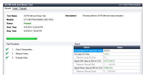
Figure 30 ASTM Drift and Noise Test – Results
