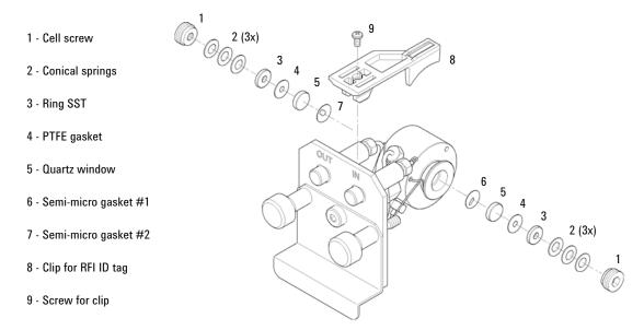
Figure 47 Semi-micro Flow Cell
