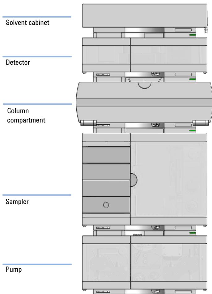
**Figure 17** Single stack configuration (bench installation, example shows a multisampler)
