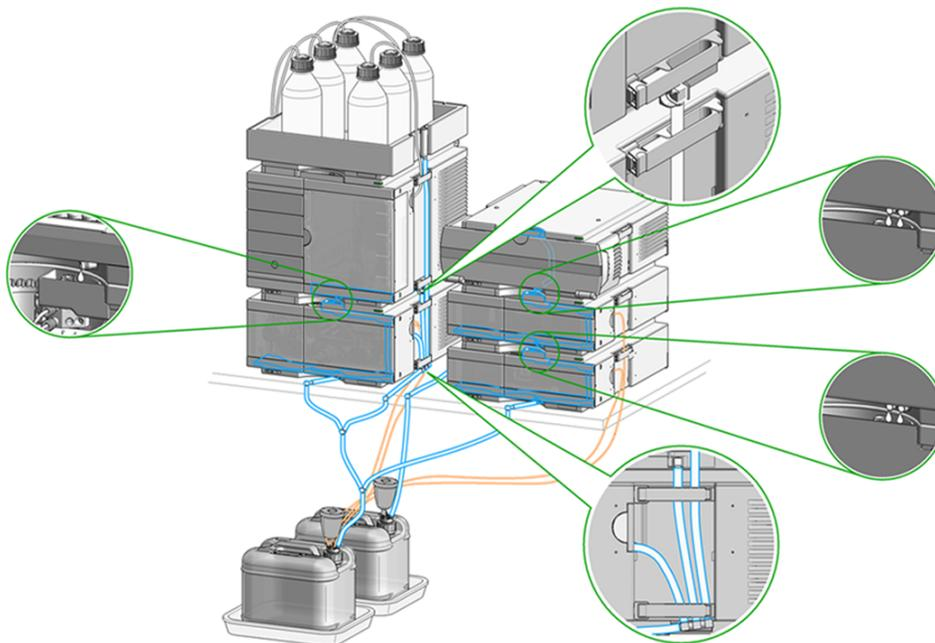
**Figure 23** Infinity II Two Stack Leak Waste Concept (bench installation)
