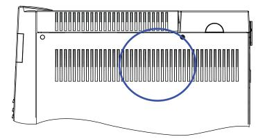
Older GC: LEDs visible through side panel.
