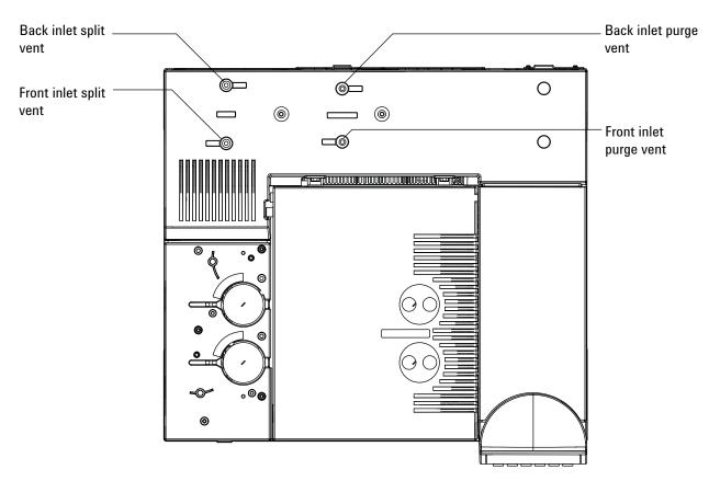
To measure split vent or septum purge flows, attach the flowmeter to the appropriate tube. Remove the GC pneumatics cover to access the back inlet exhausts.
