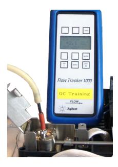
7 Place the flowmeter tubing over the flow-measuring insert to begin measuring flows.
