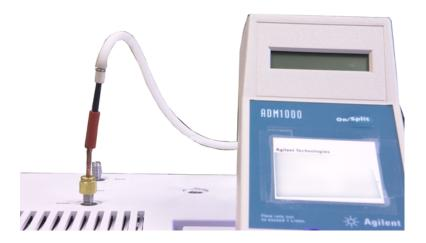
• The septum purge is a 1/8-in tube. Use the red rubber adapter shown to measure flows.
