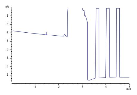
After a flameout, the GC will try to ignite the flame three times. The GC tries to reignite whenever the detector output falls below the **Lit offset** setpoint, regardless of whether or not the flame was extinguished. (In a very clean system, the baseline output may be less than 2 pA.)
