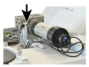
**5** Connect the flowmeter to the flowmeter adapter to measure flow rates.
