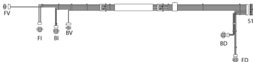
The FI and BI connectors are for inlets; FD and BD are for detectors. FV and BV are two-conductor connectors mounted on the top left edge of the GC near the inlets. They supply 24 VDC to various accessories.
