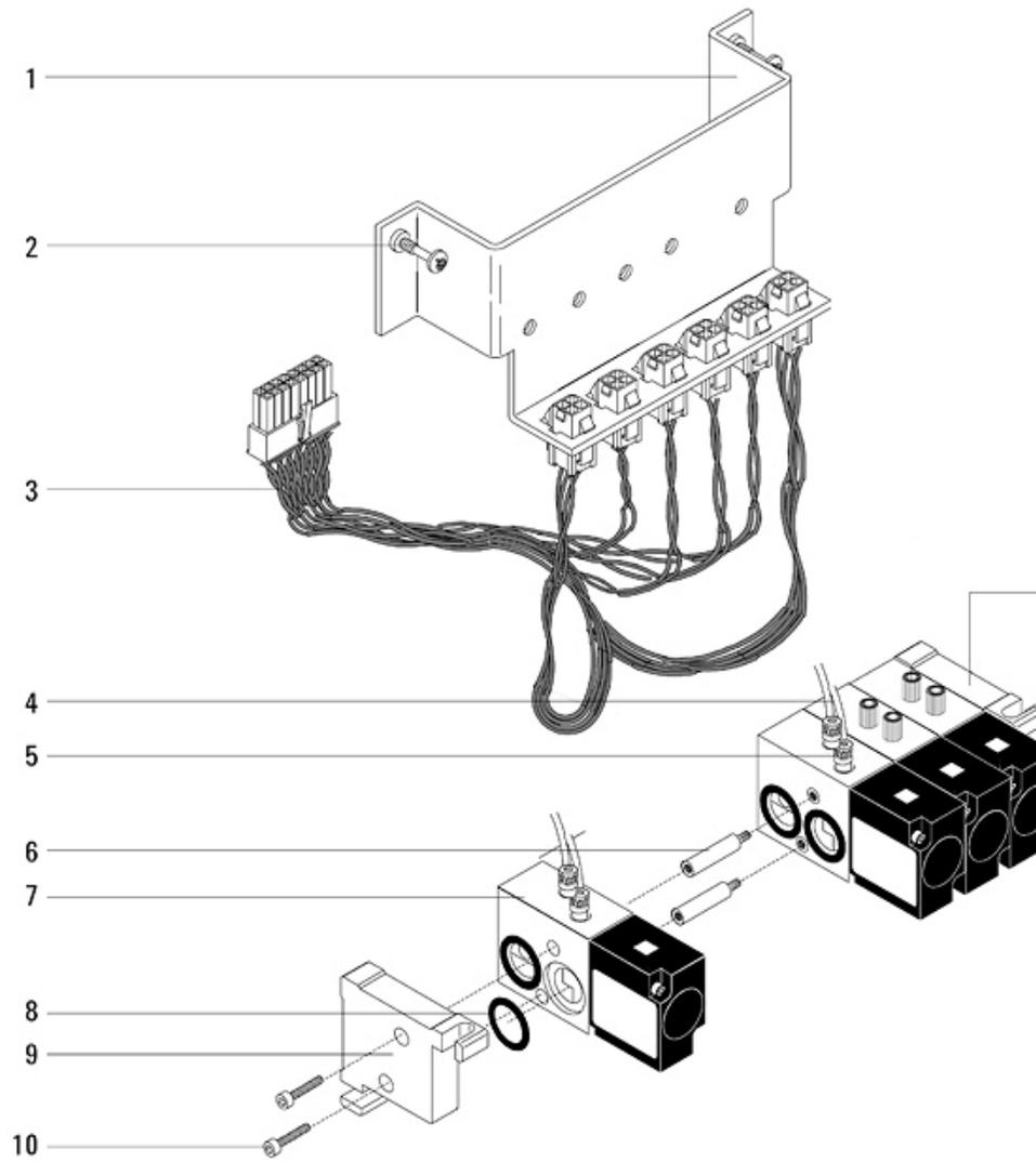
**7890A Valve actuator assembly (1 of 2)**
