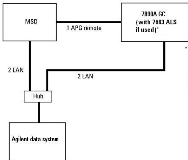
\* The 7683 ALS controls the injection to the G2913 injector tray port.
