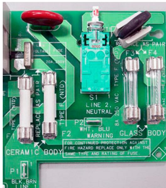
See the table below for the part numbers. When replacing both the glass and ceramic fuse types, always replace them in pairs.
