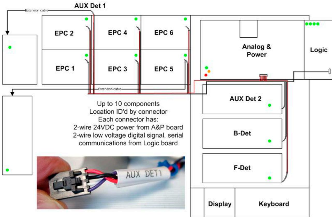
The red and black wires on the buss provide power to the module. The black wire is ground. The red wire is switched, unregulated +24 VDC. All of these wires plug into the Analog and Power Board. The white and colored wires provide serial communications between the Logic Board and the module.
