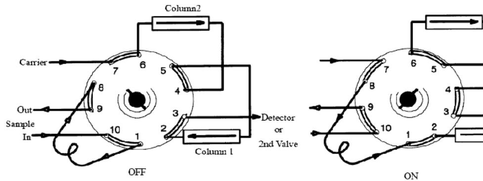
**Column Selection with Backflush to Vent, Option 806 or 836**
