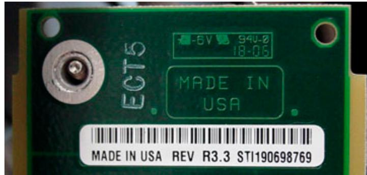
In some rare occasions, the board ID number or manufacturing date is not programmed into the board's EEPROM. In these cases, the GC will post an exception or a "bad checksum error." In this state, the detector is not usable.
