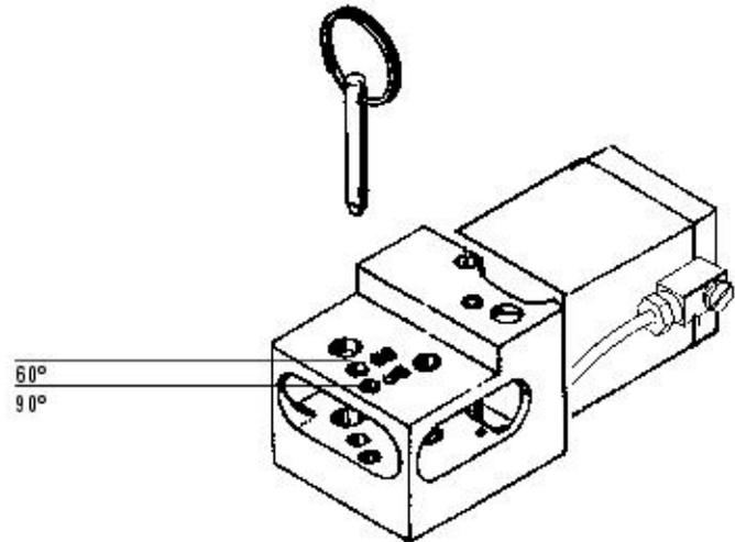
*Mounting the actuator on the valve box*
