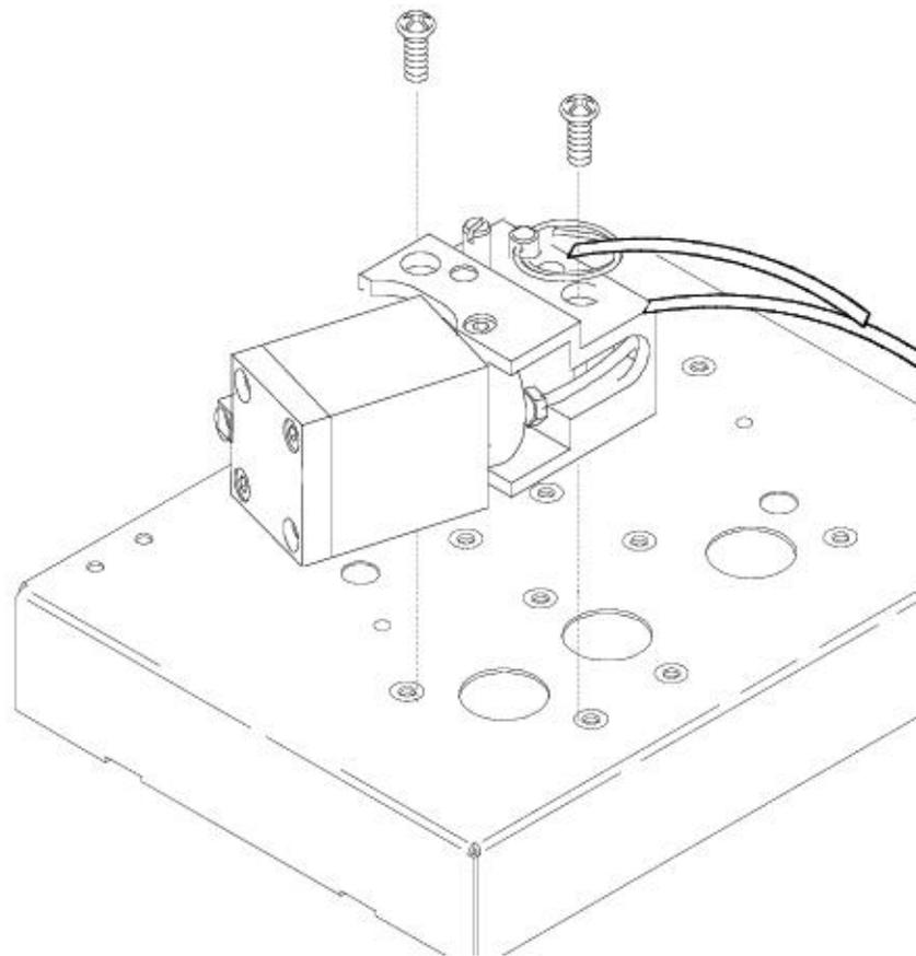
***Engaging the actuator drive shaft with the valve***
