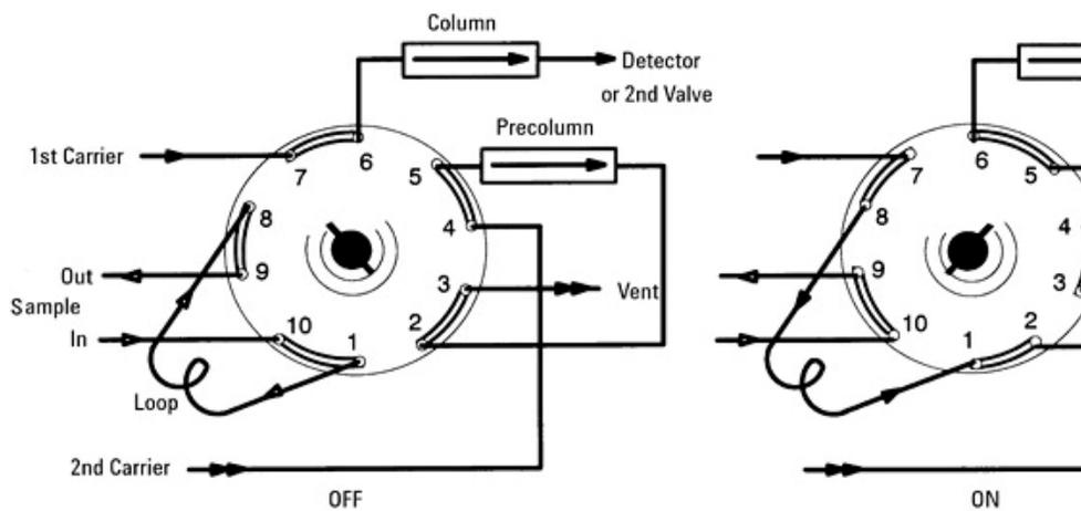
Gas Sampling with Backflush of Precolumn to Vent, Option 801 or 831
