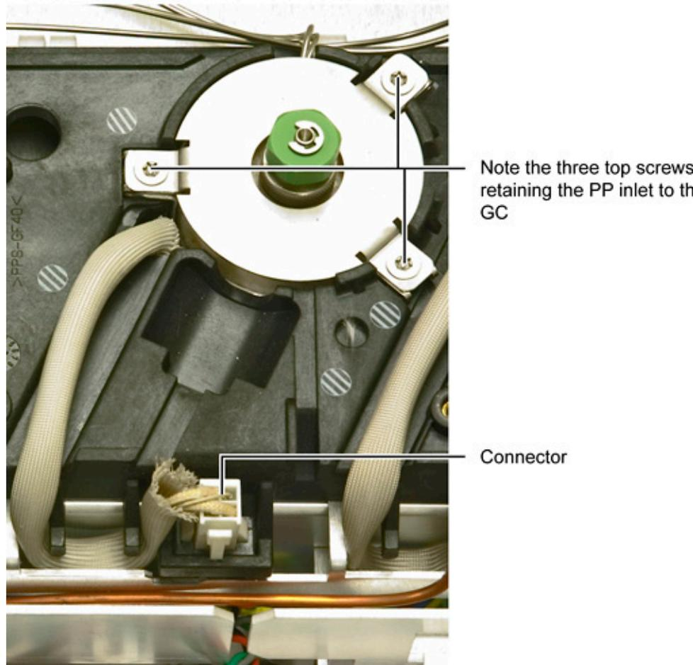
If the EPC module is disconnected, the inlet can be removed and replaced.
