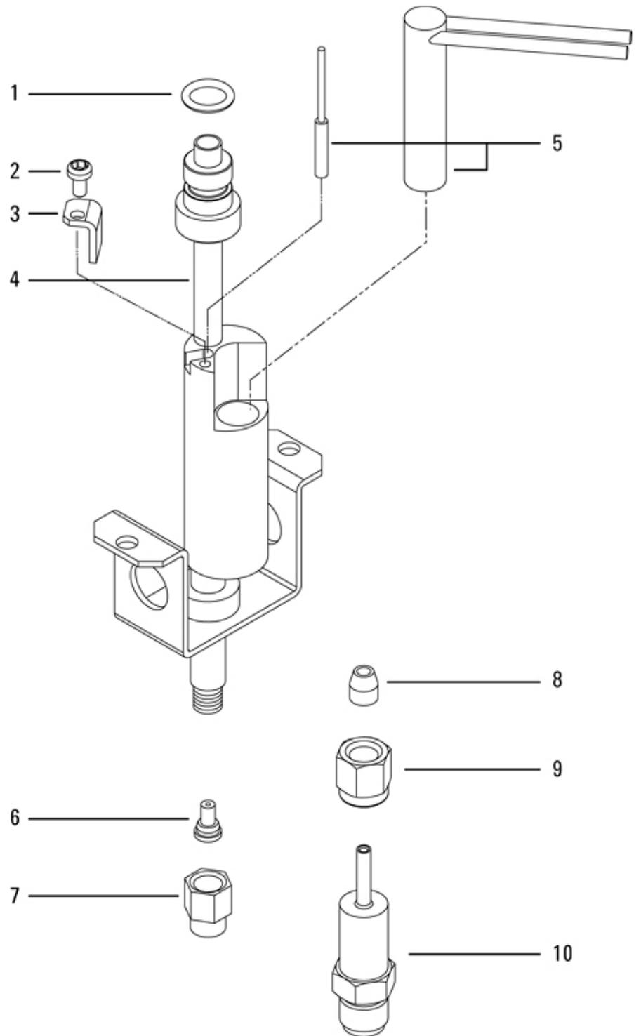
**FPD ignitor and heat shield assembly parts**
