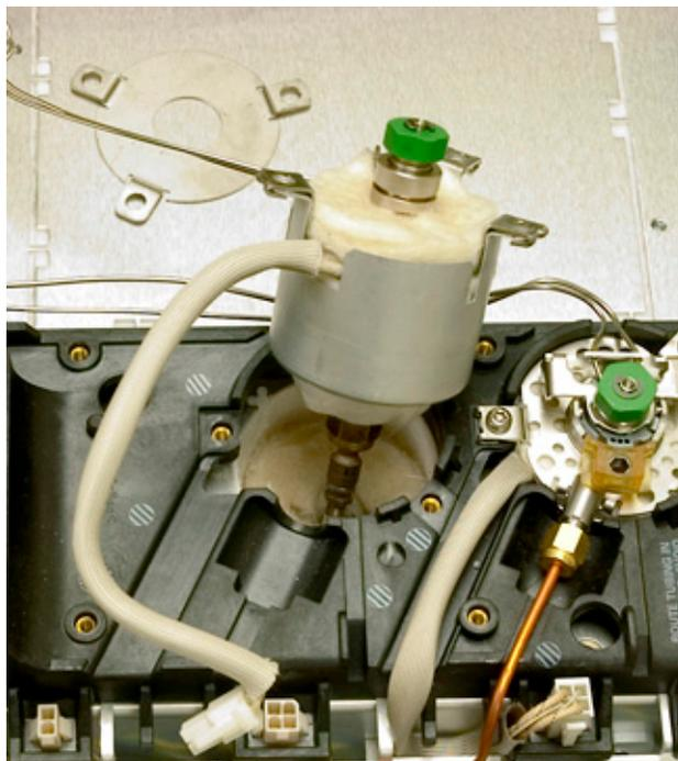
This housing is designed to accommodate a variety of Agilent inlets.
