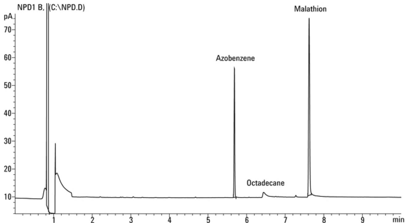
3396B or 3396C or 3397A integrator sample conditions with analog input [GC Analog output, Range 0]
