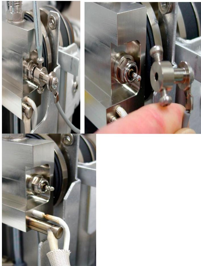
The heater/sensor assembly for the dual FPD attaches with a screw.
