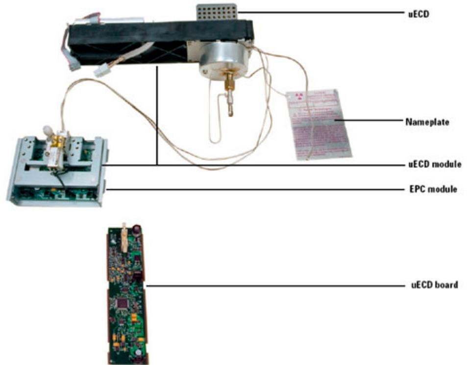
**Microcell Electron Capture Detector (uECD)**
