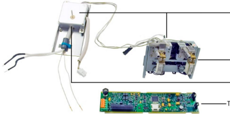
**Thermal Conductivity Detector (TCD)**
