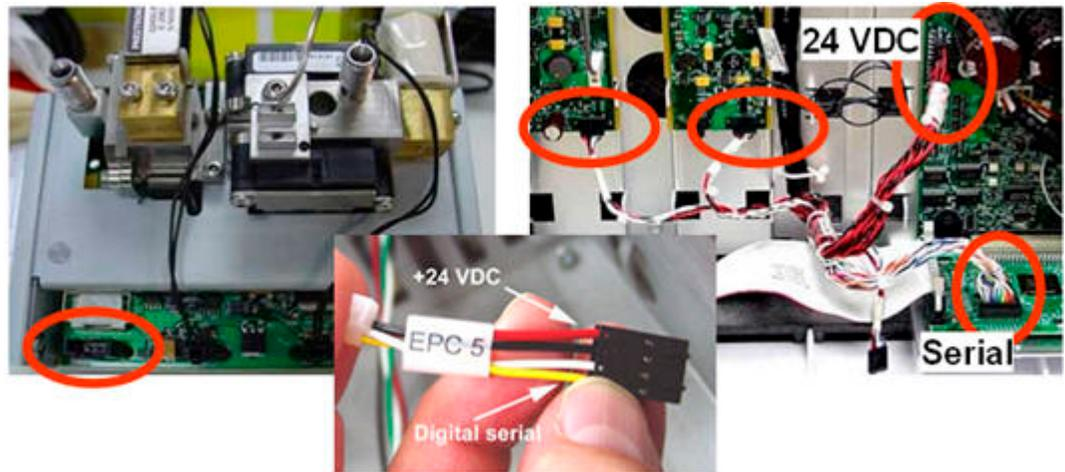
There are 2 extension cables for the GC modules of the 3<sup>rd</sup> detector:
