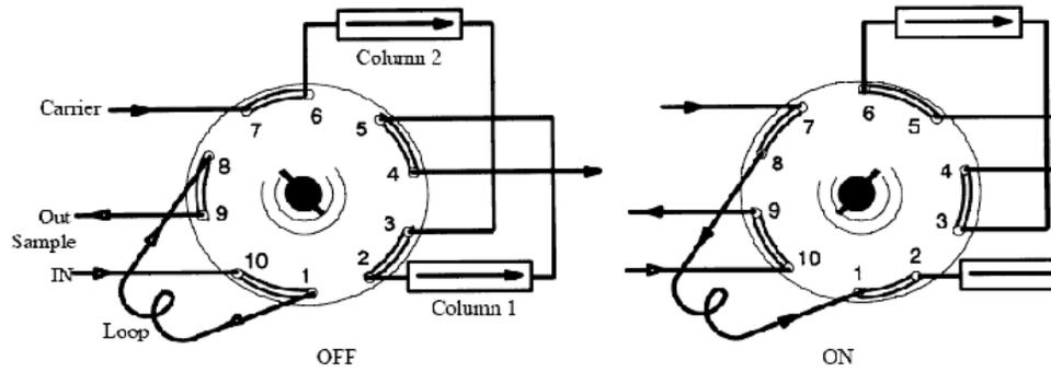
**Gas Sampling with Sequence Reverse and Backflush of Column 1, Option 805 or 835**
